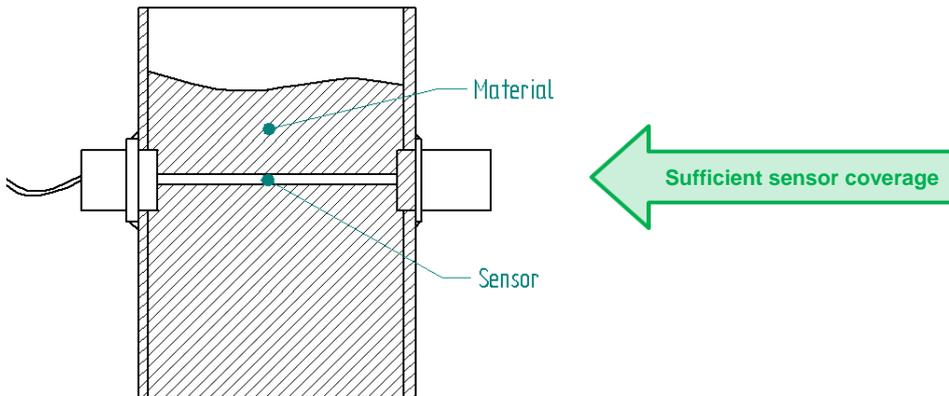
Fig. 19 Sufficient material coverage of the moisture sensor PCE-MWM 240B
