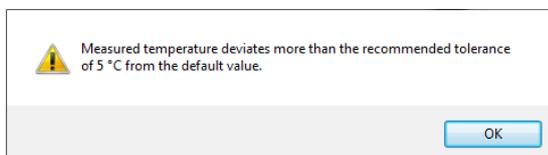
Fig. 45 Warning if measured temperature of recorded date exceeds threshold
