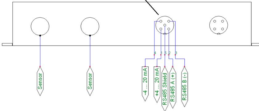
Fig. 30 Pin assignment for signal output
