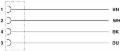
Fig. 22 Wiring diagram
