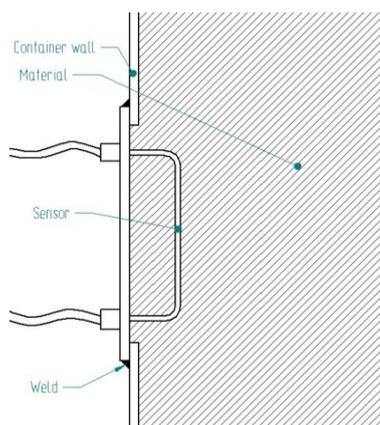
Fig. 8 Installation with welds
