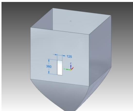
Fig. 11 Dimensions of the rectangular cut-out
