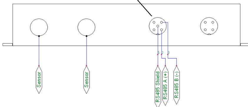
Fig. 32 Pin assignment for serial port RS-485
