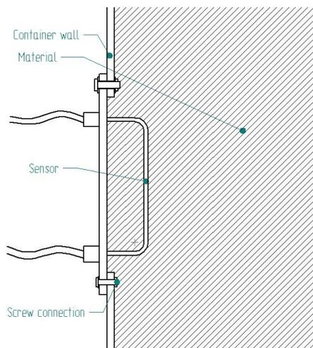
Fig. 10 Installation with screws
