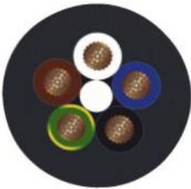
Fig. 29 Core identification code
