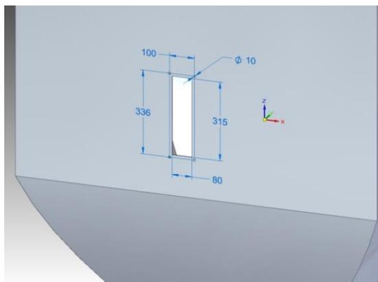
Fig. 7 Dimensions of the rectangular cut-out
