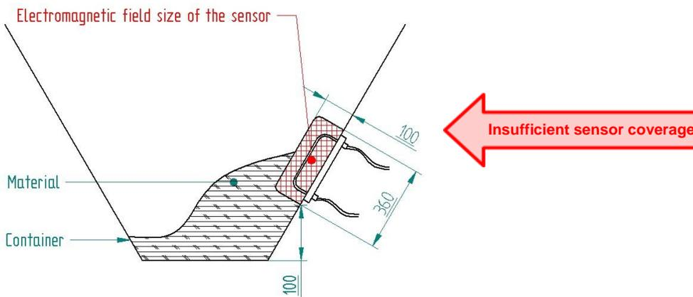
Fig. 15 Insufficient material coverage of the moisture sensor PCE-MWM 240A
