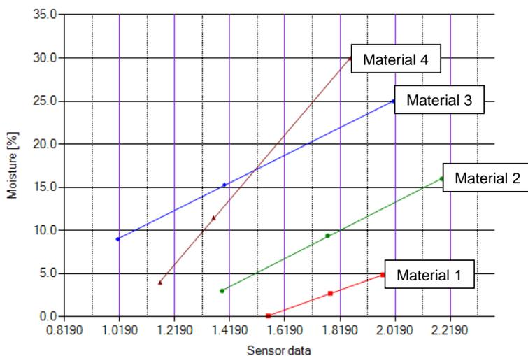
Fig. 33 Calibration curves for different material
