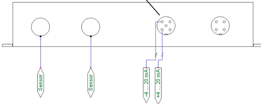
Fig. 31 Pin assignment for analog output
