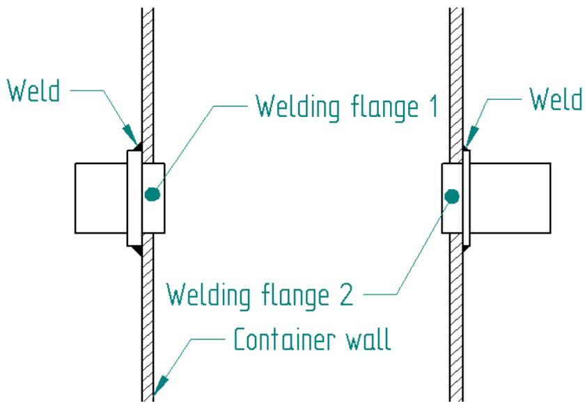
Fig. 18 Installation of the moisture sensor PCE-MWM 240B
