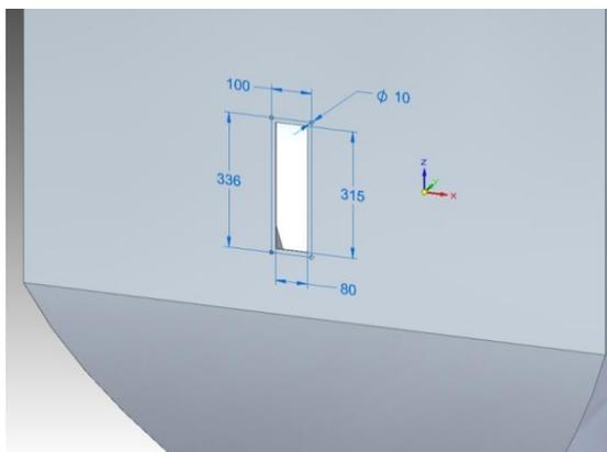
Fig. 9 Dimensions of the rectangular cut-out
