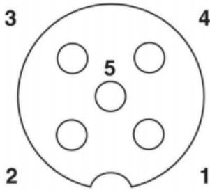
Fig. 28 Pin assignment
