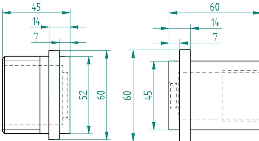
Fig. 17 Dimensions of the welding flanges
