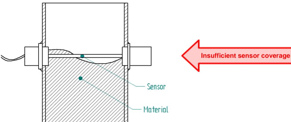
Fig. 20 Insufficient material coverage of the moisture sensor PCE-MWM 240B
