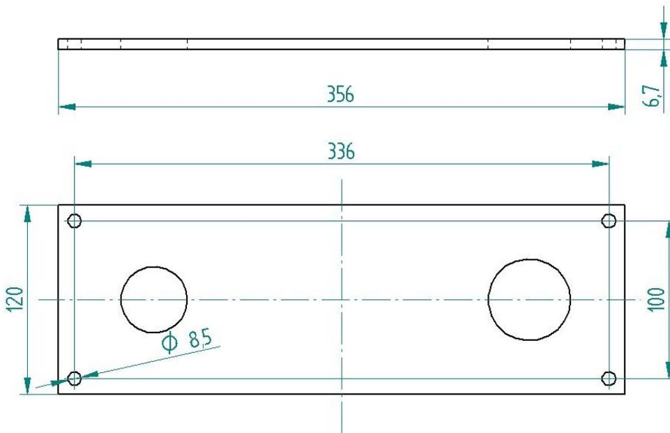
Fig. 6 Dimensions of the base plate of the moisture sensor PCE-MWM 240A
