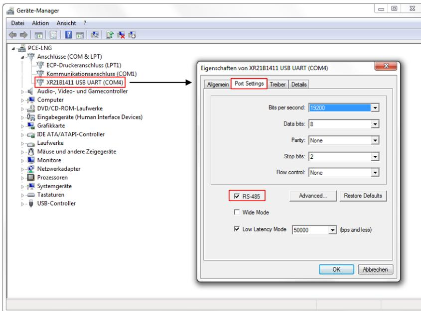
Fig. 35 Configuring RS-485 Adapter
