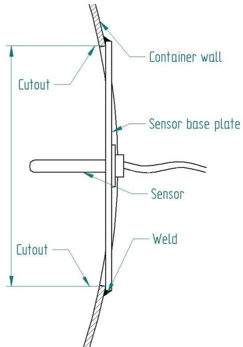
Fig. 13 Installation on a curved surface
