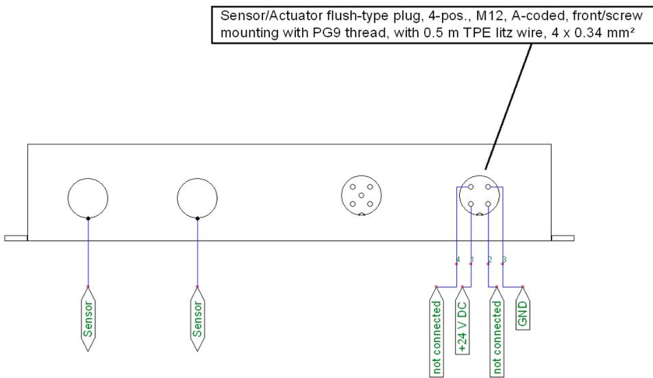
Fig. 25 Pin assignment for power supply
