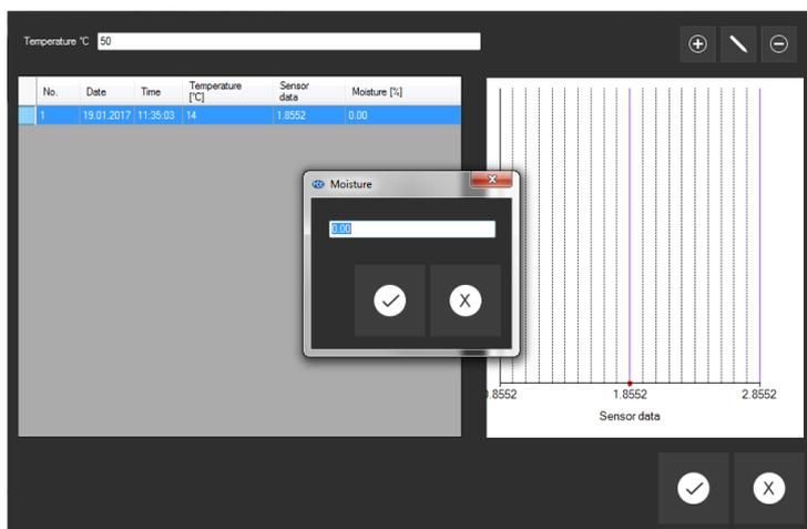
Fig. 47 Assign moisture to sensor data
