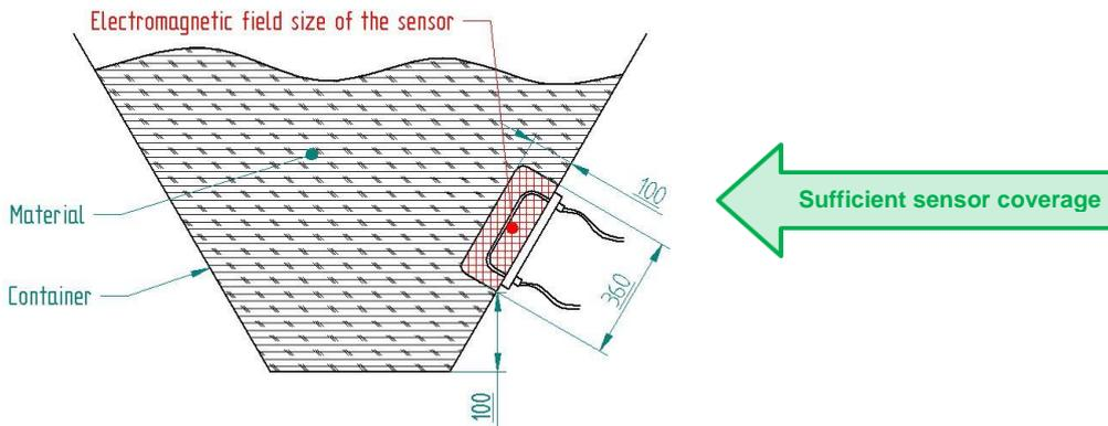
Fig. 14 Sufficient material coverage of the moisture sensor PCE-MWM 240A
